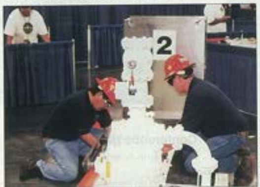
Guy Moriguchi (left) and Clifford Kiger of the KOA Nitrifiers (Hawaii Water Environment Association) break down and rebuild a 3-in. (76-mm) Gorman-Rupp self-priming centrifugal pump during the Maintenance event.
