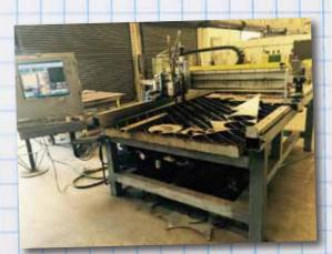
BUILDING A PRECISION CUTTING TOOL FROM SALVAGED PARTS ENABLES THE VILLAGE CREEK WATER RECLAMATION FACILITY (FORT WORTH, TEXAS) TO MAKE THE CUSTOM PIECES IT NEEDS FOR REPAIRS. VIllage Creek Water Reclamation Facility
