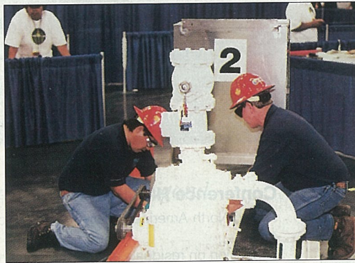
Guy Moriguchi (left) and Clifford Kiger of the KOA Nitrifiers (Hawaii Water Environment Association) break down and rebuild a 3-in. (76-mm) Gorman-Rupp self-priming centrifugal pump during the Maintenance event.
